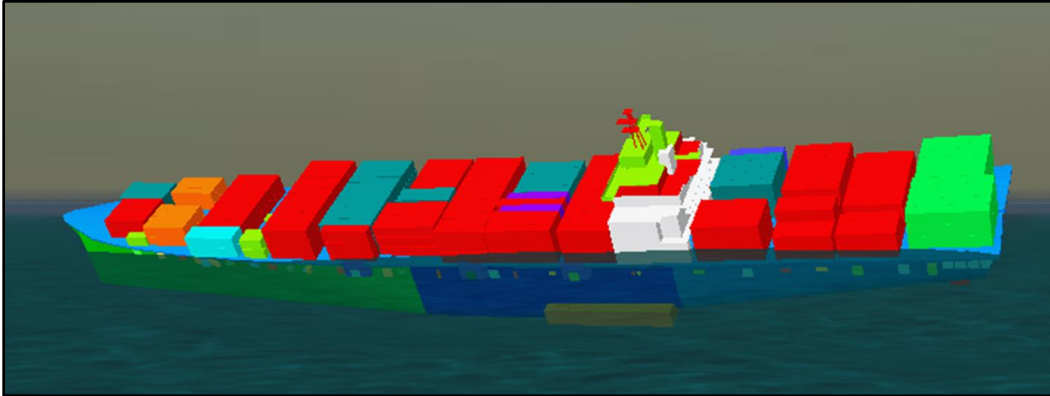
Figure 61. El Faro rolling about a 15° to 18° static heel with waves or green water reaching ventilation openings after propulsion loss. (Screen shot at extreme position from CSRA video simulation)
