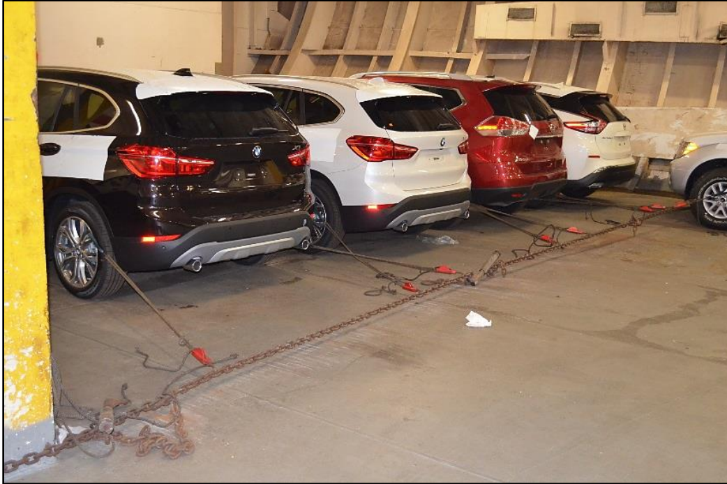
Figure 22. Two automobiles lashed to one length of chain. (Photo from hold 5 of El Yunque )
