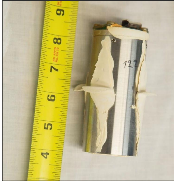
Figure 16. Inner VDR capsule assembly after removal from outer capsule.
